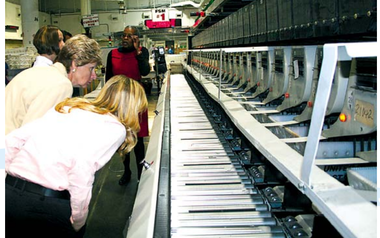
During the Plant Tour, attendees take a closer view of the Flat Sorter Machine, which sorts barcoded flat mail by zip code for delivery
