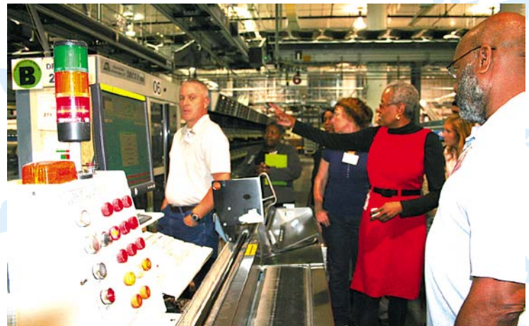
The tour continues with a look at the DBCS (Delivery Bar Code Sorter) which sorts barcoded letter mail by zip code for delivery
